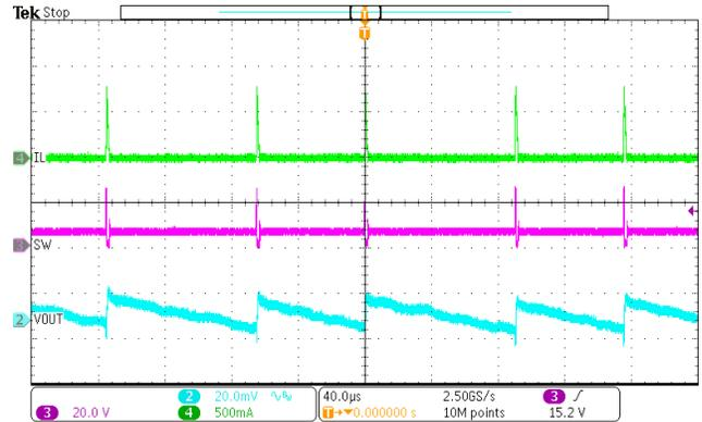
Figure 17. SW node Waveform and Output Ripple
