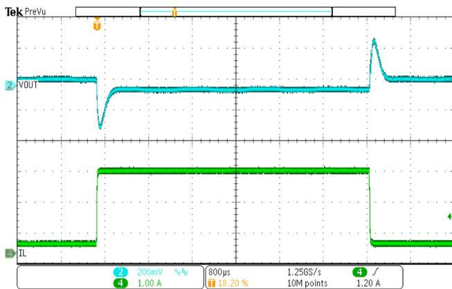
Figure 20. Load Transient
