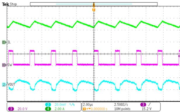
Figure 16. SW node waveform and Output Ripple
