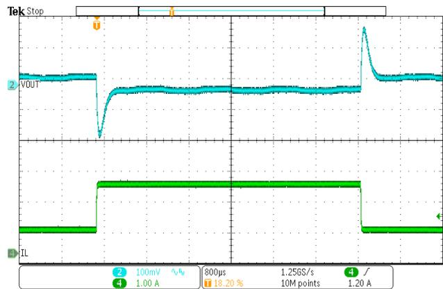
Figure 21. Load Transient
